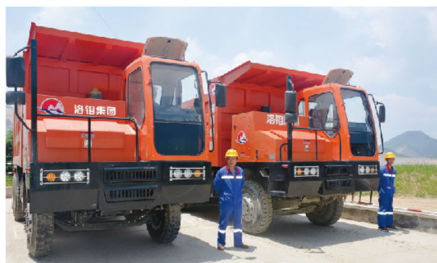
In 2018, we have successfully developed electric driverless mine truck operations, which have passed the inspection of the National Mining Machinery Quality Supervision and Inspection Center. Radar, camera, and sensors provide multiple omnidirectional sensing, vision-based target detection and recognition and moving target trajectory. Under this system the truck can plan a route and give feedback in real time so that automatic driving can be realized, driving safety can be improved and the occurrence of casualties can be reduced.
