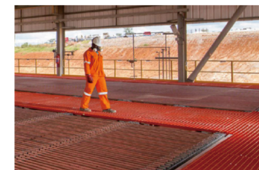
▲ A worker in the electrowinning facility at our TFM operation. Open-sided buildings and personal protective equipment are examples of controls used to reduce employee exposure to potentially noxious air quality in this facility.
