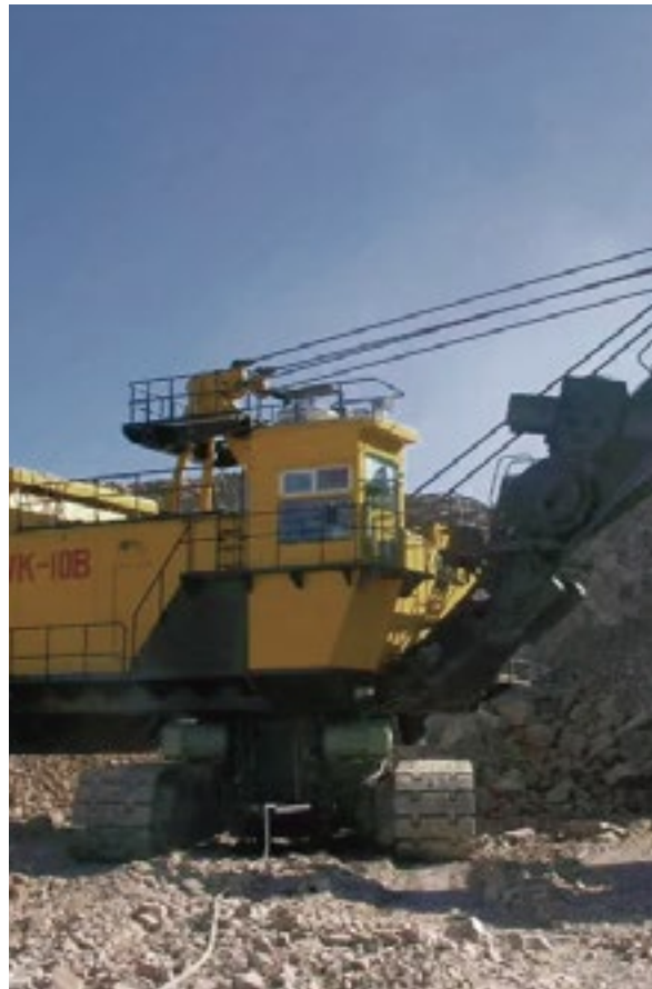
Our China site uses electric excavators to reduce the use of fossil fuels.
