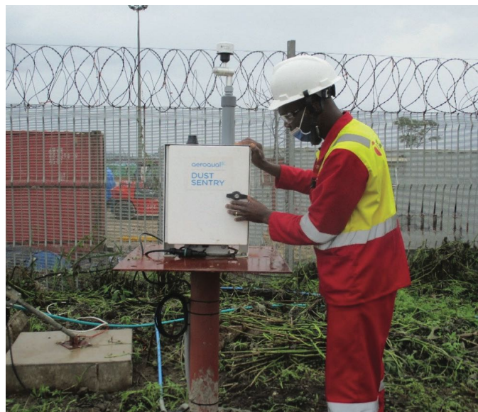
In 2022, we upgraded our on-site PM10 monitoring equipment to enable automatic, online monitoring in real time
